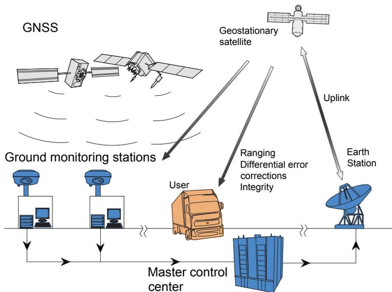
Assisted-GNSS (A-GNSS) is a method used mainly in smartphones to improve positioning performance and especially the time needed to compute the receiver position when positioning is activated: i.e. Time To First Fix (TTFF). A-GNSS is based on providing data with the help of mobile network services, e.g. a rough estimate of location or satellite orbital data, to the receiver via cellular network.
