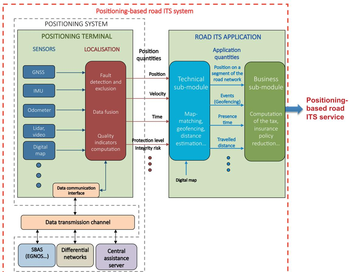
A GNSS-based positioning terminal, potentially merging other sensors or sources of data, provides a position (3D, 2D or 1D) expressed in an absolute reference system, such as WGS84. However, depending on the processing done in the terminal and the chosen data stream, it can also provide velocity (3D or 2D vector), speed (the magnitude
