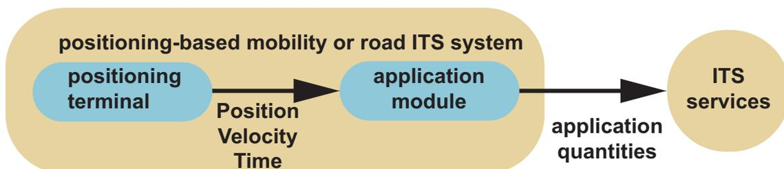
For instance, the system Personal Navigation Device (PND) comprises a positioning terminal (the GNSS receiver chipset with its antenna) and an application which performs map-matching, attributes retrieval and user information generation through the human-machine interface. The service is the guidance to the driver.
