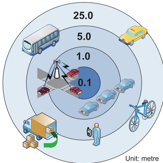
From these examples, the availability of services depends to a great extent on the accuracy and reliability<sup>3</sup> a positioning system can provide. The more accurate and reliable the positioning information is the more stringent service it can support.
